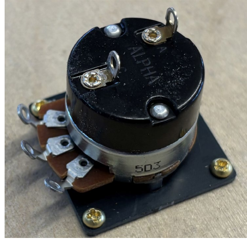
Figure 15 - Pot Adapter Plates and Screws. In rare instances you'll have to mount the pots to the inside of the cabinet using these plates and screws instead of mounting them in the metal chassis.
