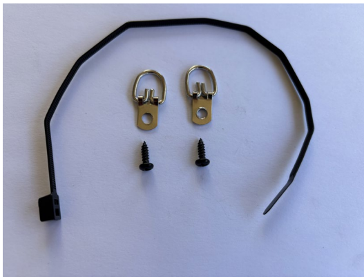
Figure 14 - Large zip tie, D-Rings, and screws are used to secure the power supply to the cabinet.
