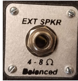
FIGURE 3 - EXTERNAL SPEAKER JACK. THIS IS A BALANCED (UNGROUND) CONNECTION. DO NOT CONNECT TO A GROUND-CONNECTED MONITOR.
