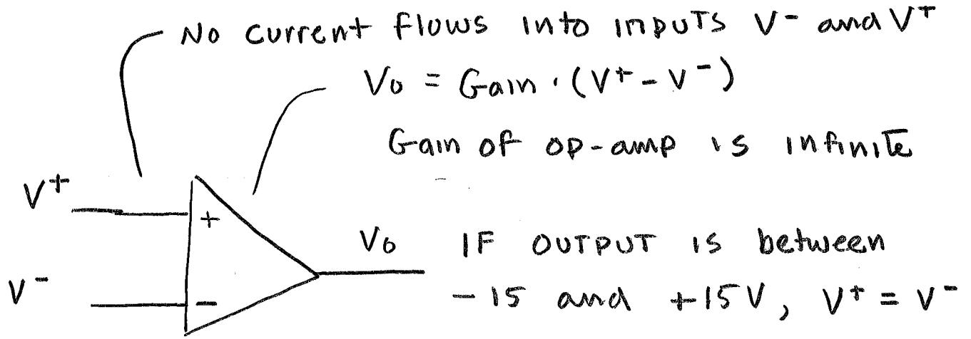
Gain of op amp is infinite. What is the gain of this circuit?
