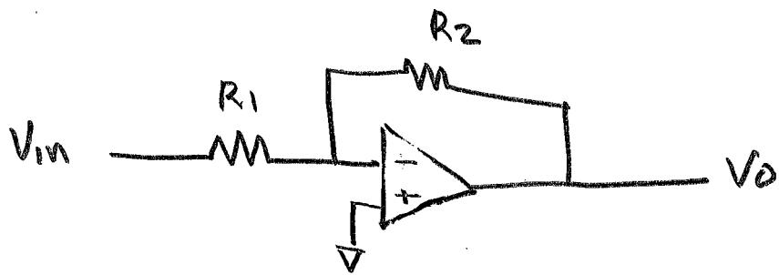
KCL at inverting terminal: (No current into  $V^-$ )
