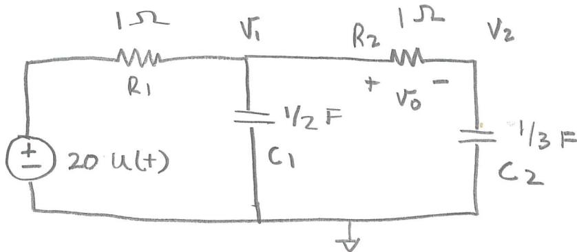
Find  $v_0$  (+) Hint: (first find  $v_1$  and  $v_2$ )
