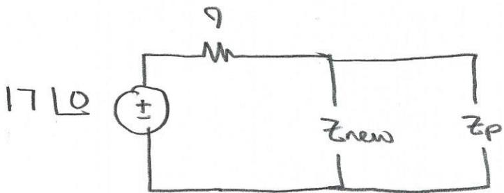
$$\begin{aligned} \frac{Z_P}{n^2} &= \frac{Z_c Z_R}{Z_c + Z_R} \times \frac{1}{n^2} = \frac{\frac{Z_c}{n^2} \times \frac{Z_R}{n^2}}{\frac{Z_c}{n^2} + \frac{Z_R}{n^2}} = \frac{Z_c Z_R}{Z_c + Z_R} \times \frac{\frac{1}{n^2}}{\frac{1}{n^2}} \\ &= \frac{Z_c Z_R}{Z_c + Z_R} \times \frac{1}{n^2} \end{aligned}$$
