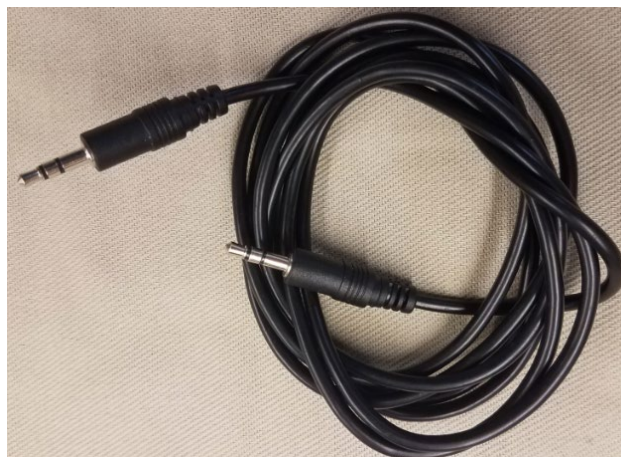
Figure 6 - Standard 3.5 mm to 3.5 mm stereo cable with male connectors on both ends.
