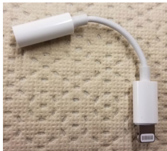
Figure 5 - Lightning to 3.5 mm Headphone Jack Adapter. You will need this if you test your SEA-310 with an iPhone 7 or newer.
