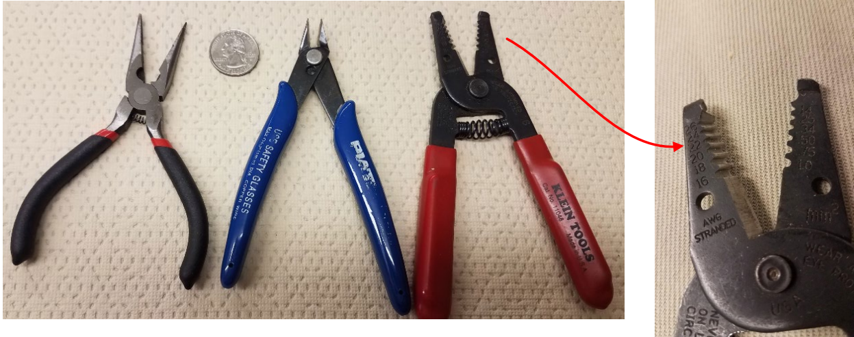
Figure 2 - Needle-nose pliers, diagonal cutters, and wire stripper. The quarter is shown so you can see the size of these tools. The numbers on the wire stripper show where to put different stranded or solid wire sizes so they'll be stripped correctly. Make sure your stripper can strip stranded wire gauges from #18 to #24. Find a video to show you how to use the wire stripper.
