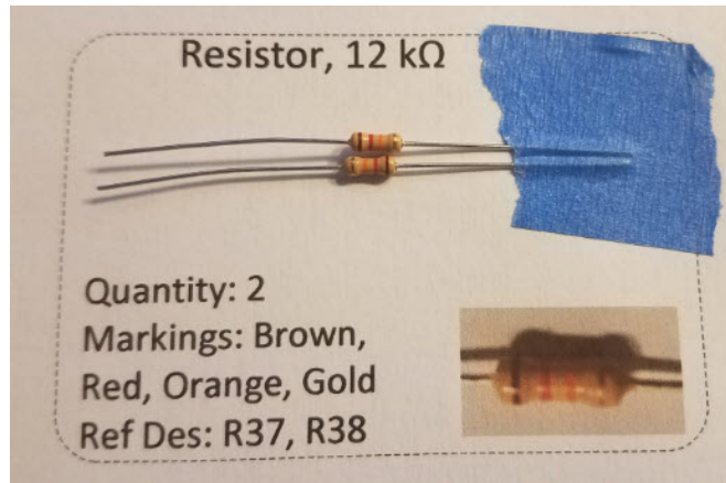
Figure 13 - Tape the components to the inventory sheets using painter's tape. Don't block the text because you'll need to see it when you stuff the board. Use Table 8 on Page 64 to determine where to put these parts on the PCB.
